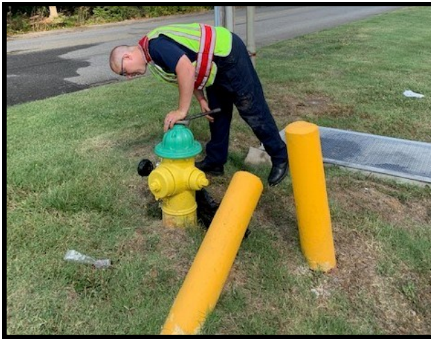
Pictured Above: Engineer Lee Paine Checking static pressure (PSI) on hydrant
